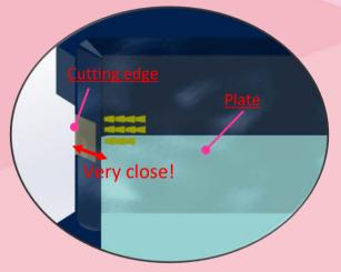
The area around the blade has a simple shape. This makes it possible to approach the wafers and glass plates close to the blade, making the collection easier.
